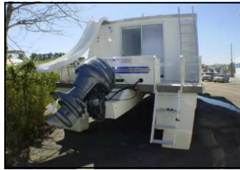
Aft end of the 12' wide V-40' & V-43' (sitting on white blocks). Order with a single- or double-outboard installation. Slide & ladder optional.
